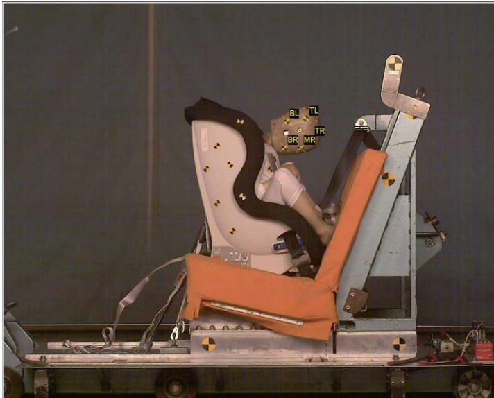
The orientation and 3D movement of the surveyed dummy head is measured by TEMA Classic 6DoF with single camera view.
